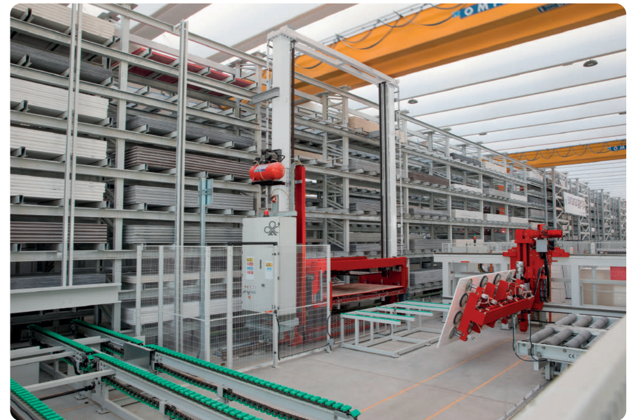
Double-mast picker stacker crane with suction cups (marble sector)
