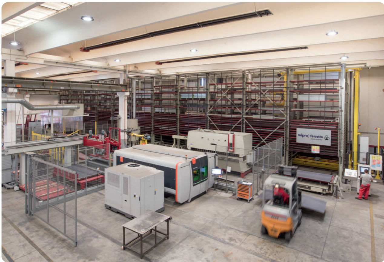
Automated storage system for sheet metal
