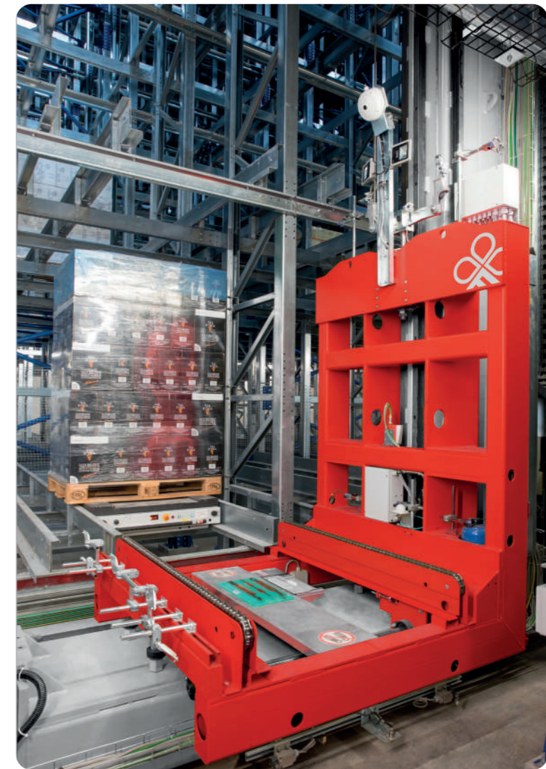
Multi-depth automated storage system for pallets
