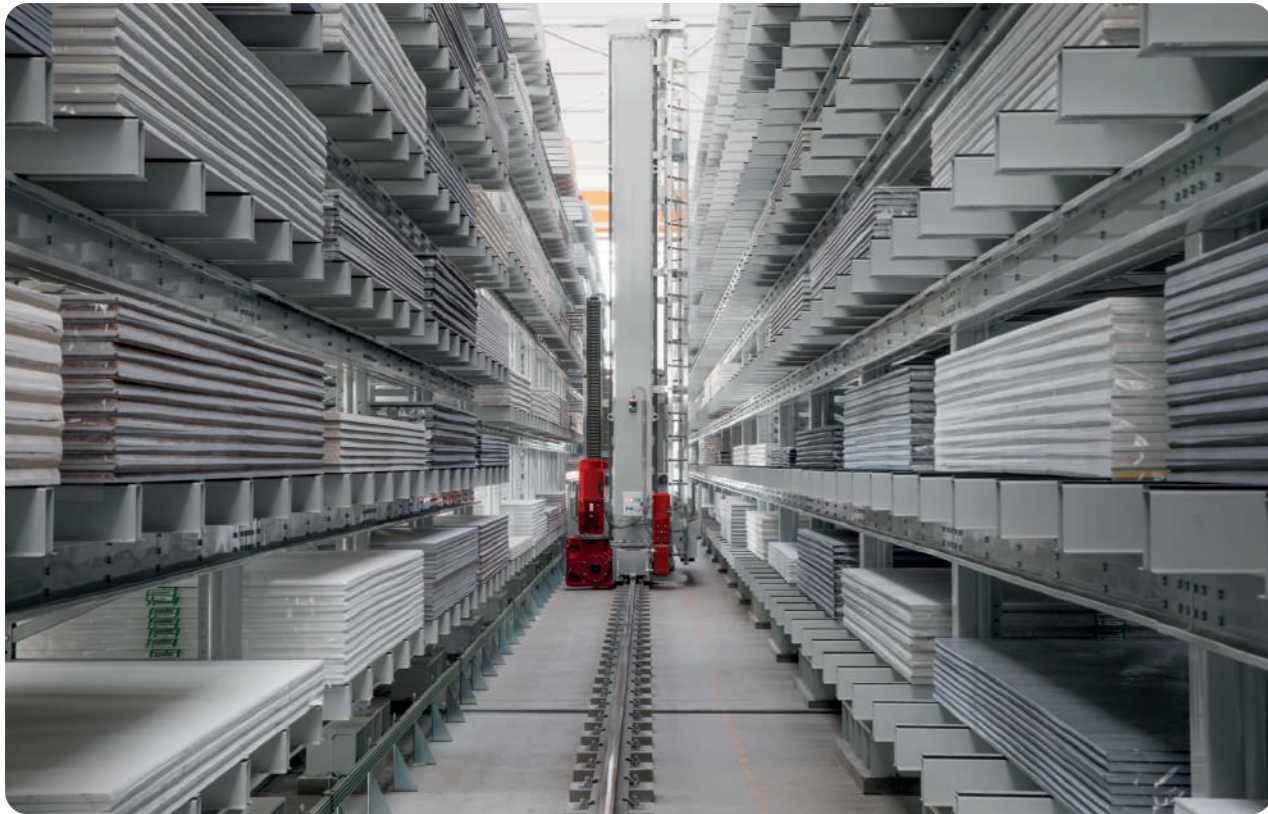
Automated storage system for marble slabs
